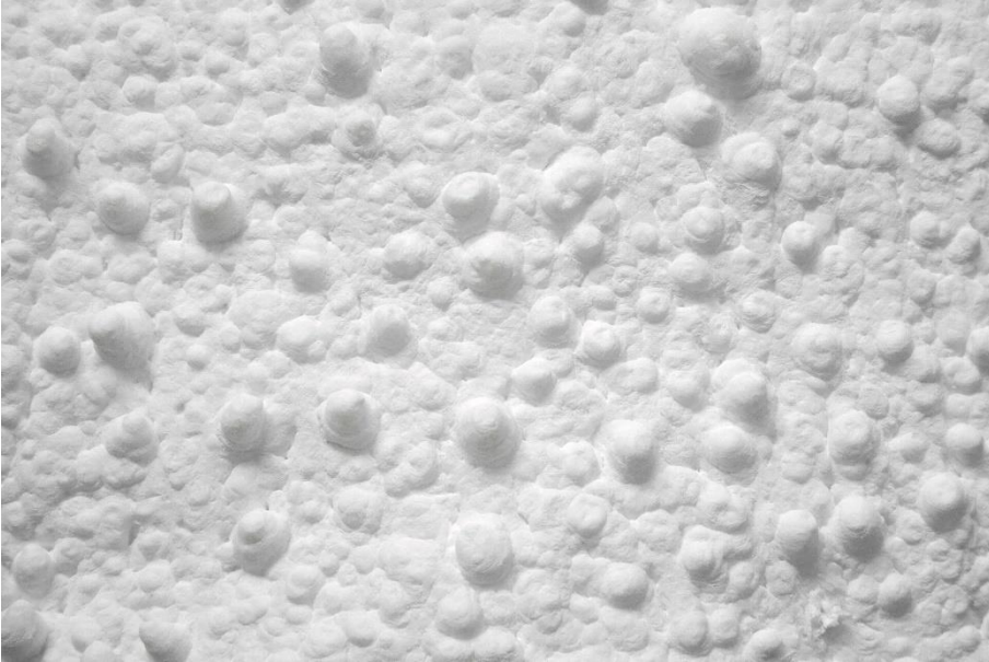
Clariant's Intumescent coatings foam and expand when exposed to high heat, forming an insulating char that protects the underlying material. © Clariant
