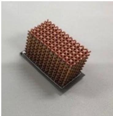
Example 2: Power devices for EVs need heatsinks. A small sized heatsink component is test-developed for each device. Prototype heatsinks printed in pure copper on the Concept Laser M2.
