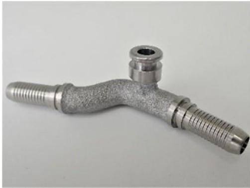
Example 4: Thin wall pipe of a motor sports engine unit. Ti-6Al-4V is printed into a thin wall pipe with a wall thickness of 0.8 mm using EBM. It was put into practical use as an engine pipe for motorsports after passing a 1-MPa high pressure test.
