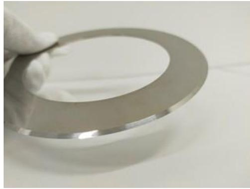
Example 1: Using CoCrMo (a corrosion resistant, hard-to-work material, alloy), an industrial slitter knife has been printed using EB to make a cutting tool with optimal hardness and toughness for a wide variety of applications from resin films to metal thin films, electrodes, as well as foodstuffs.
