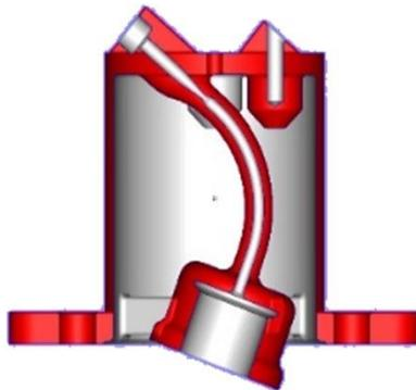
Attitude control injection nozzle manufactured in Ti-6Al-4V on EBW technology for KOUNOTORI, the unmanned cargo transfer spacecraft for the International Space Station.
