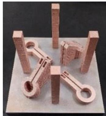
Example 3: Newly developed thin wall, pure copper pipes for induction heating (IH) coils. High-frequency induction quenching coils made of pure copper, a material that is difficult to process by precision bending or welding, are integrally formed using EB technology. A method for forming thin wall pipes with a wall thickness as thin as 0.5 mm is currently under development.
