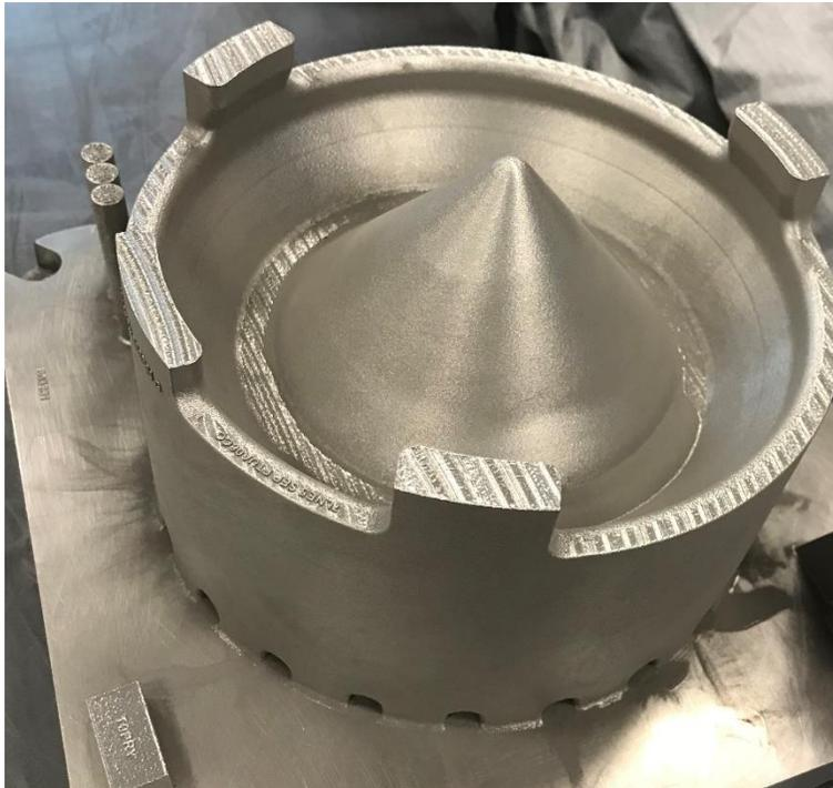
Additively manufactured, cobalt-chrome sump cover for F110 engine. Produced on a GE Additive Concept Laser M2 machine at the GE Additive Technology Center in Cincinnati, as part of collaboration with the US Air Force's Rapid Sustainment Office (RSO). (Photo: GE Additive, GEADPR049)
