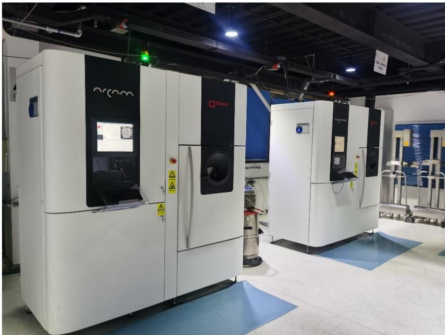
Arcam EBM Q10plus machines installed at AK Medical's Beijing facility.
