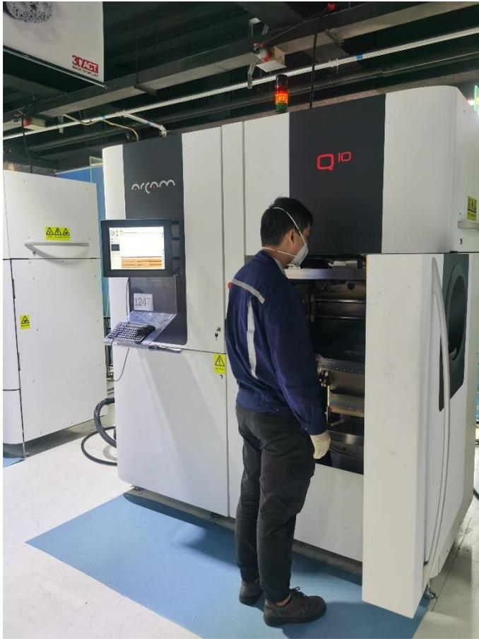
Operator using Arcam EBM equipment at AK Medical's Beijing Facility.
