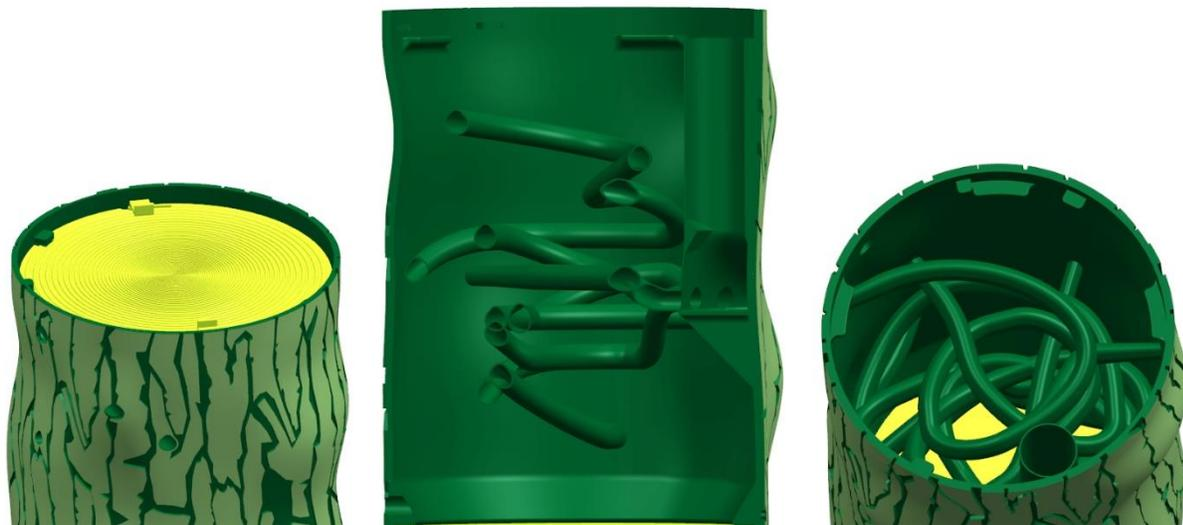
CAD models of metal 3D Printed cricket feeder for Cincinnati Zoo.
